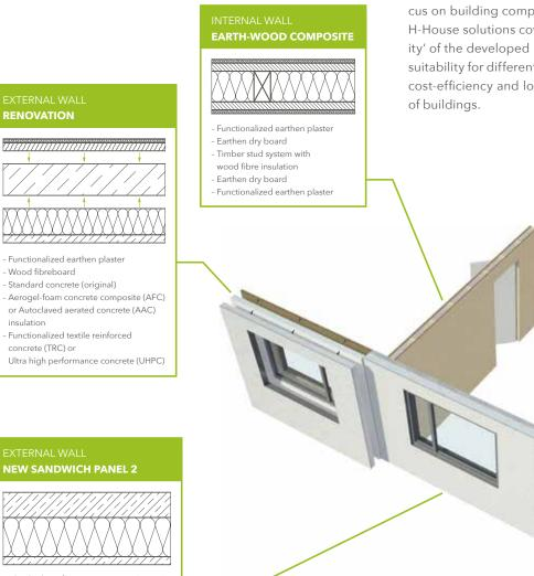
Ultra high performance concrete (UHPC) - Autoclaved aerated concrete (AAC) insulation Surface functionalized UHPC
