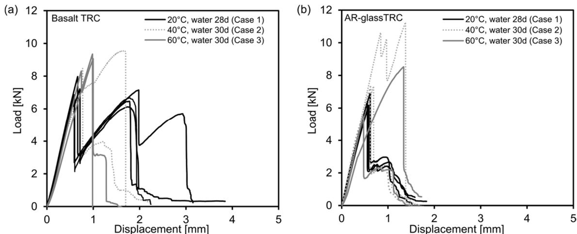
Figure 4. Results from the uniaxial tensile tests: basalt TRC panels (a) and AR-glass TRC panels (b).
