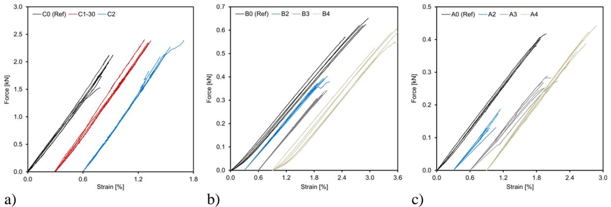
Figure 3. Results from the direct tensile tests: carbon textile (a), basalt textile (b) and AR-glass textile (c). For visualization, the initial strain was shifted 0.3%-units relative to each previous case.
