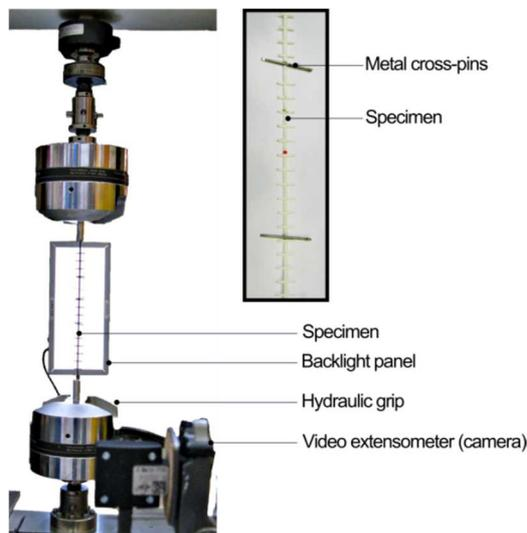
Figure 1. Direct tensile test setup applied in Study 1 (from [8]).
