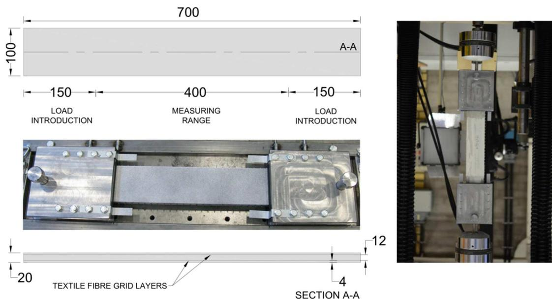
Figure 2. Panel dimensions and clamp detail (left) and test setup for uniaxial tensile test (right).
