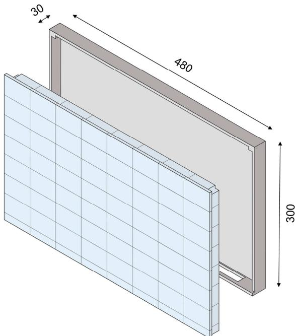
Fig. 1. Non-load bearing façade element for refurbishment (size in cm).
