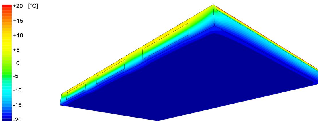
Fig. 5. Temperature distribution of the façade element.
