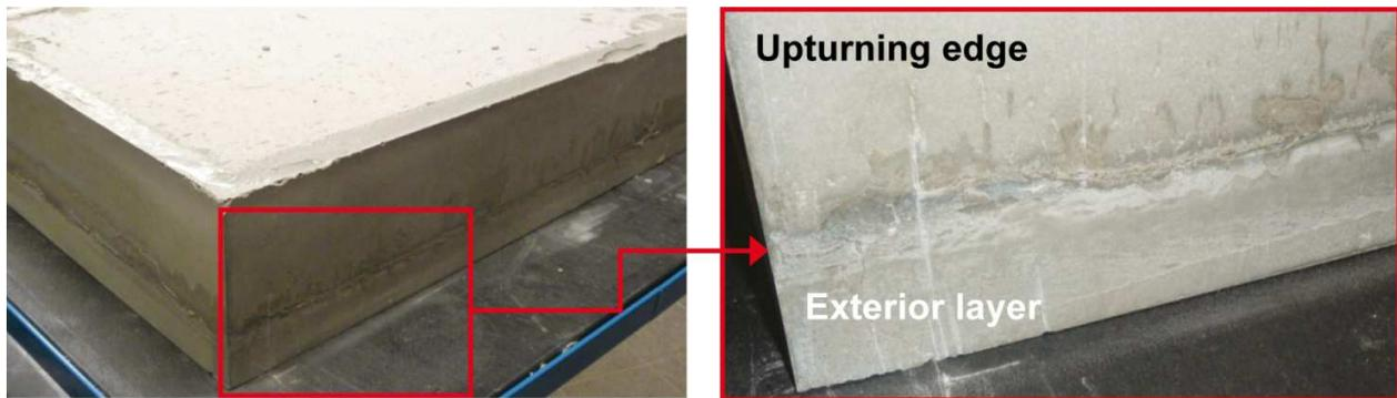
Fig. 4. UHPC box manufactured with the two-step procedure: joint between exterior UHPC layer and upturning edges.
