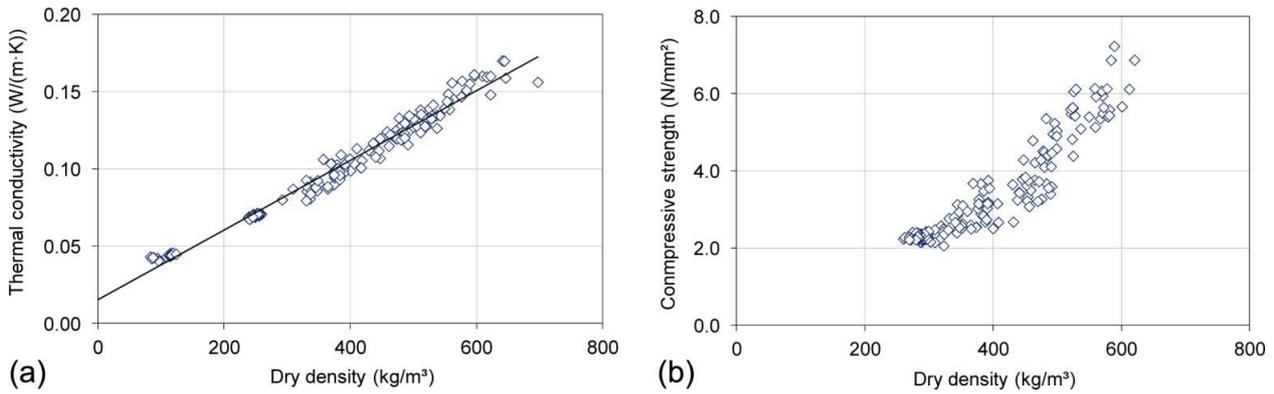
Fig. 2. Correlation between AAC dry density and: thermal conductivity (a); compressive strength (b).
