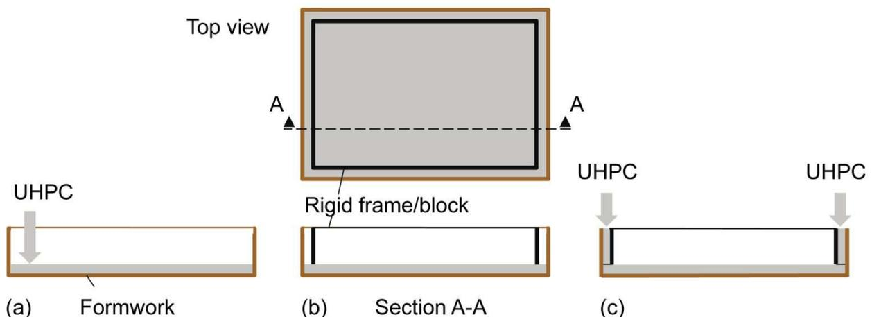
Fig. 3. Procedure for two-step production of box-shaped UHPC elements: (a) cast of exterior layer; (b) placement of a rigid frame as internal formwork on hardened exterior layer; (c) cast of upturning edges.
