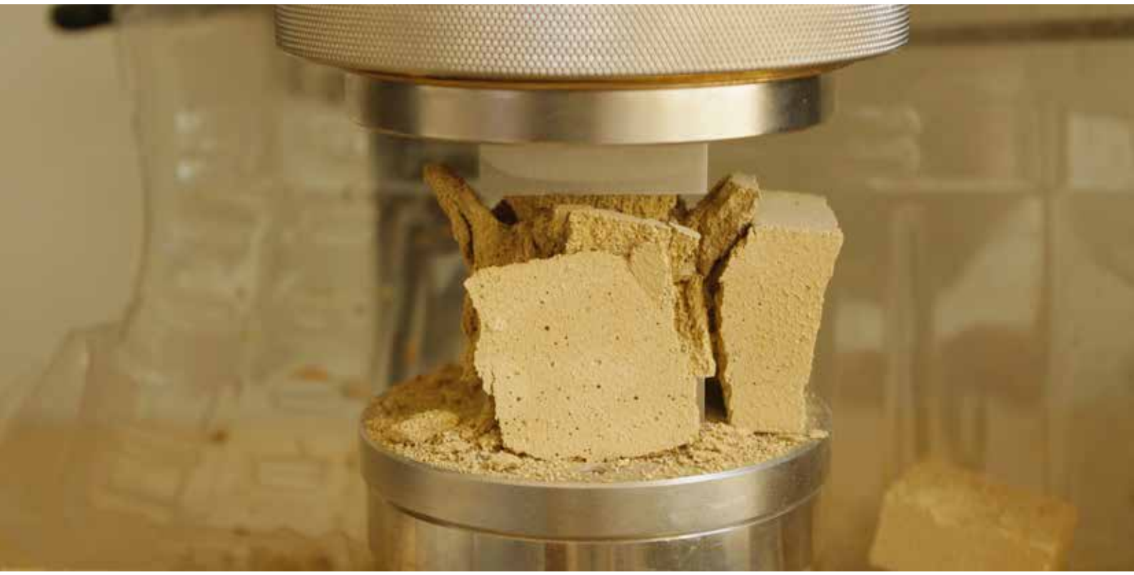
▲ Mixing process of aerogel modified earth plaster ▶ Microscopic image of aerogel modified earth plaster specimen ▼ Compressive strength test of modified earth plaster specimen
