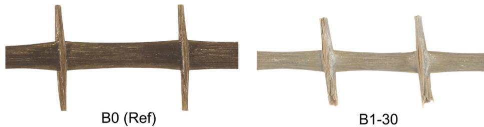
Fig. 5. Visual comparison between pre- (B0) and post-immersion (B1-30) for the basalt product.
