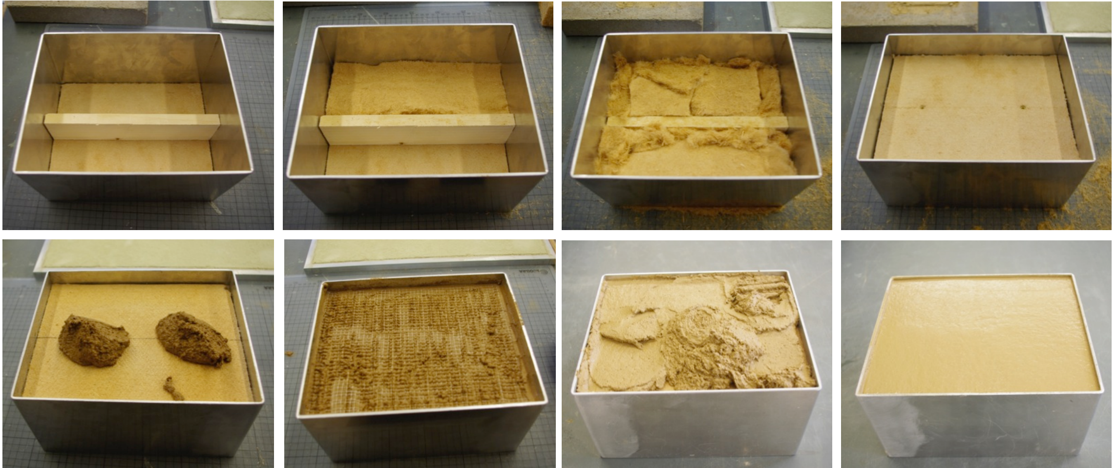
Wall build-up: earth plaster (straw) + earth adhesive + wood fibreboard + wood fibre insulation
